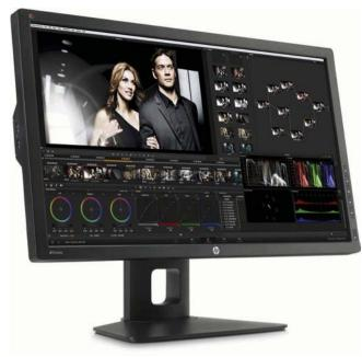
to 4096x2160 pixels), which is then downsampled for viewing on the available 2560x1440 native panel. Framerate (vertical frequency) is limited in this case to 24 progressive frames per second though.
