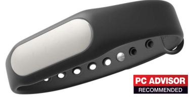
with ultra-low power consumption (less than one fifth of similar devices), a Dialog DA14580 lowenergy Bluetooth 4.0 chip and a super-thin 8mm 41mAh battery. To charge the battery you'll need to remove the Mi Band core and attach it to a proprietary USB cable.
